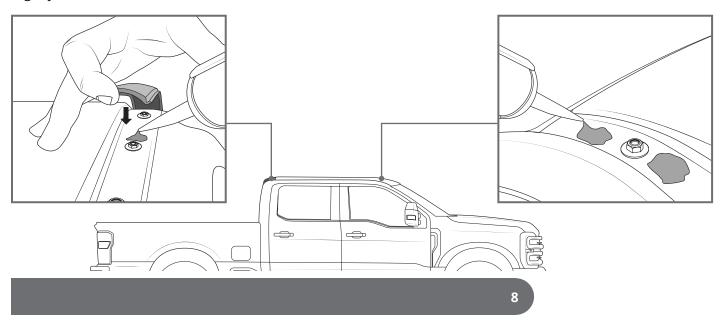
Using the sealant as an adhesive, place the cut out front and rear sections of the ditch back into place.
