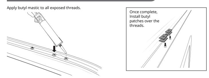
Apply butyl mastic at the front and rear of the gutter. The rear gutter molding can be lifted slightly for access.
