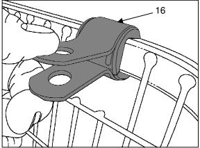
42. Place a pivot saddle (16) over each of the pivot saddle bushes then push the ends together.
