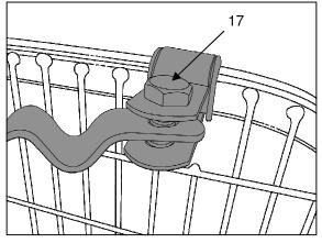
43. Place the correct strap in between the pivot saddle ends then place a hex screw (17) through the saddle and strap.
