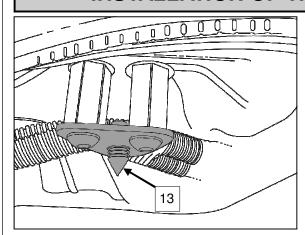
24. Screw a marking pin (13) into one of the roof brackets with approx. 8mm protruding.
