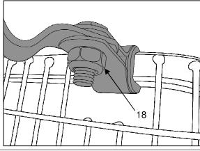
45. Place a nyloc hex nut (18) onto each of the hex screws then tighten until the strap is firm in saddle but can still be pivoted.
