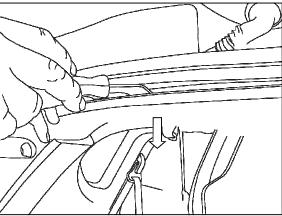
12. Using a suitable trim removal tool remove the 3 trim clips securing the back edge of the roof lining in place.
