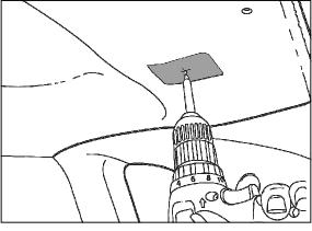
28. At the marked locations from steps 26/27 carefully drill a pilot hole through the roof lining. (Use of a drill stop set at 10mm is recommended)
