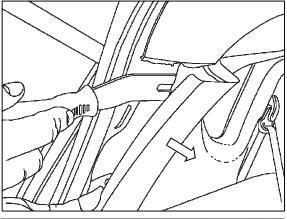
11. Using a suitable trim removal tool unclip the rear pillar trim tops as far forward as the rear windows.
