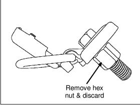
5. Unscrew the hex nut located on the back of the 'D' anchors and discard. Nut will be replaced with a tube spacer from the kit.
