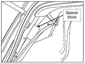
13. Place a spacer block or similar behind the rear pillar trims as shown.
