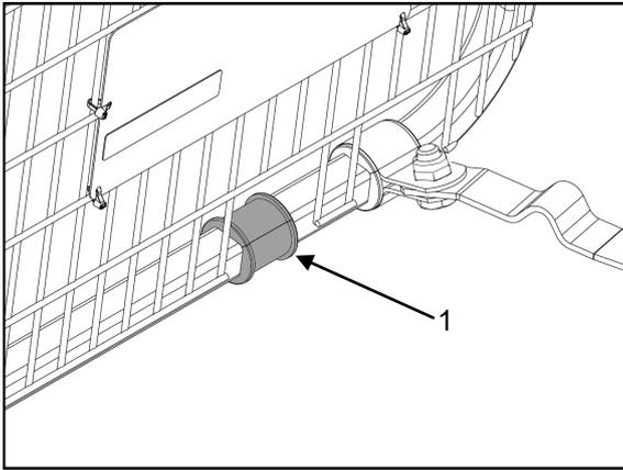
2. Place a saddle bush (1) over the cargo barrier frame as shown.
