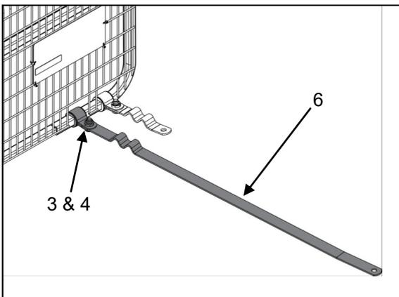
4. Place a bottom front position strap (6) in between the saddle as shown then secure with an M10 bolt and nut (3 & 4).
