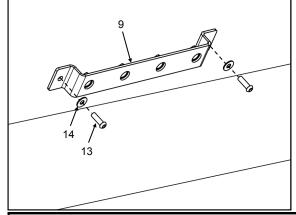
16. Secure the bracket ASM (9) to the vehicle using the M6 button head screws (13) and flat washers (14) as shown.
