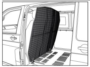
24. Position the cargo barrier ASM behind the front seats in the vehicle as shown.
