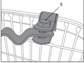
22. Place the correct strap in between the pivot saddle ends then place a hex screw (5) through the saddle and strap.
