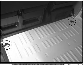
17. Find the two 'D' anchors located behind the front seats in the vehicle.
