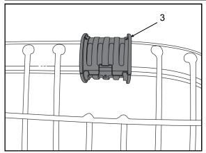
20. At each of the cut outs in the mesh on the perimeter of the cargo barrier, place a pivot saddle bush (3) as shown.
