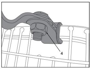
23. Place a nyloc hex nut (4) onto each of the hex screws then tighten until the strap is firm in saddle but can still be pivoted.
