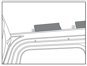
4. For single sliding door models affix masking tape to the roof panel on the RHS (drivers side), in the approximate locations shown.
