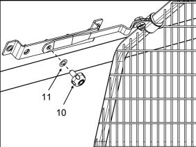
25. Secure the top straps in place using a 19mm Milbolt (10) and crinkle washer (11) as shown.
