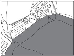
1. At the front of the cargo area place a cover sheet over the floor area to catch any drilling swarf.
