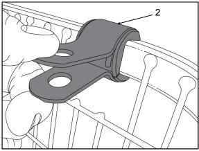
21. Place a pivot saddle (2) over each of the pivot saddle bushes then push the ends together.
