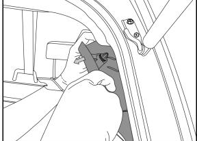
24. With the aid of a trim removal tool carefully unclip the back and top edge of the rear inner 1/4 trims. Both sides.
