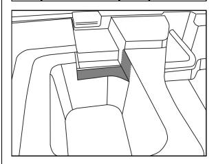
To enable the cargo area floor panel to be easily removed without releasing the bottom cargo barrier straps, the following modification to the foam floor insert should be made.
