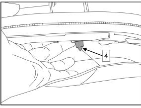
32. Screw a marking pin (4) into each of the captive nuts in roof brackets with approximately 8mm protruding.
