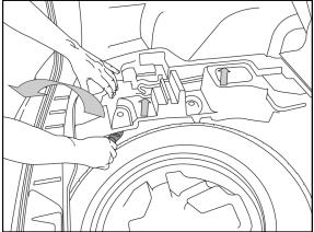
Using a trim removal tool to assist, carefully unclip and remove the styrene foam under floor inserts. Store in a safe place.
