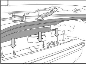
26. Using a suitable trim removal tool unclip the back edge of the roof lining allowing enough space to access the tailgate hinge securing nuts.
