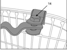
47. Place the correct strap in between the pivot saddle ends then place a hex screw (14) through the saddle and strap.
