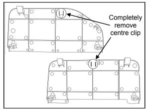
13. On the back side of both of the trim covers removed at step 5, cut away the centre clip flush to the back face of cover as shown.
