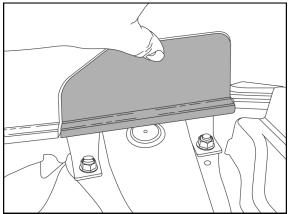
14. Carefully relocate each of the trim covers back into their home position, then apply pressure to the marking pin area until a mark is left on the back face.
