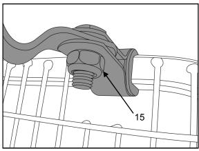
48. Place a nyloc hex nut (15) onto each of the hex screws then tighten until the strap is firm in saddle but can still be pivoted.
