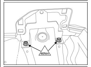
10. With the bottom brackets in position replace the flanged hex nuts removed earlier.
