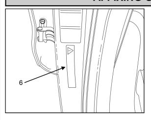
44. Clean area inside drivers door opening just below side airbag warning label as shown, using cleaning pad (5). Allow to dry then affix orange warning label (6) at that location as shown.
