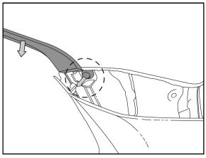
25. With the aid of a small screwdriver remove the trim clip circled, then unclip the back end of the trim above side window.
