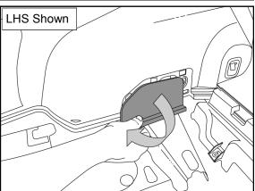
5. At the sides of the cargo area in the wheel arch area, unfasten and remove the clip on covers. Both sides. Store covers in a safe place.
