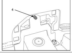
12. Screw a marking pin (4) into each of the captive nuts in bottom brackets, with just the point protruding.
