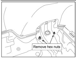
7. Using a 14mm AF socket remove the hex nuts securing the rear suspension struts in place. Both sides. Retain the nuts for reuse later.
