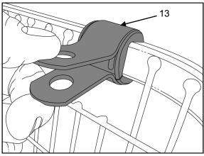
46. Place a pivot saddle (13) over each of the pivot saddle bushes then push the ends together.
