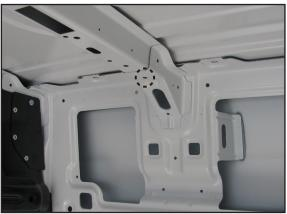
2. Find the hole shown on the first crossbeam from the front of the vehicle, on both sides.
