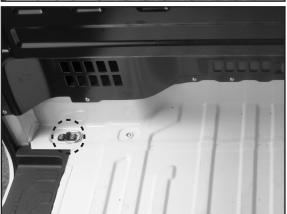
Remove the screws securing the 'D' anchors in place, and remove the 'D' anchors from the floor of vehicle. Retain for use in step 33.
