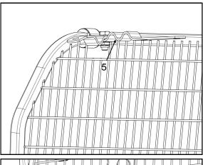
Attach a top strap (5) underneath the pivot saddle, and secure the nut back onto the screw. Tighten until the strap is firm but can still be pivoted.
