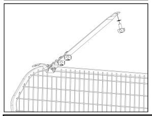
10. Secure the top straps to the top mounts at the rear of the vehicle with the Milbolts used for the rear position as shown.
