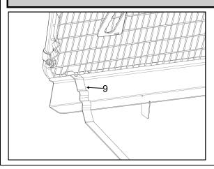
11. Remove the Milbolt and washer attached to the LHS of the lift panel ASM and place a LHS bottom strap (9) as shown.
