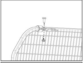
Unscrew the bolt and nut from the top strap. Leave the rear position strap in place at the moment. Discard the 20mm long saddle screws.
