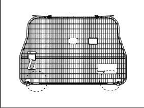
Locate the open apertures in the cargo barrier mesh at the bottom of the cargo barrier.
