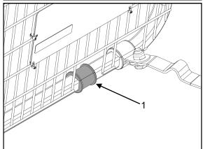
Place a saddle bush (1) over the cargo barrier frame as shown.
