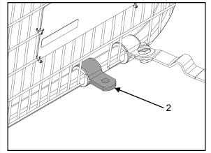
3. Place a pivot saddle (2) over the saddle bush then push the ends together.
