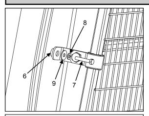
14. With a tube spacer (6) in between the side straps and the vehicle panel, secure the side straps to the existing captive nuts using hex screws (7) with spring & flat washers (8 & 9) under heads.
