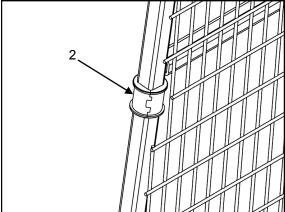
5. On the sides of the cargo barrier at each of the cut outs in the cargo barrier mesh, place a pivot saddle bush (2) over the frame and clip shut. (2 places)
