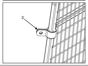
6. Place a pivot saddle (3) over each of the pivot saddle bushes then push the ends together to clamp over the bush as shown.
