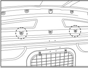
4. At the front of the cargo area near the roof line remove the screws (circled) and discard.
