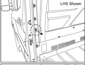
3. At the front of the cargo area remove the screw (circled) and discard. Repeat on the other side.
