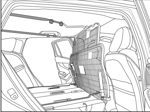
12. Fasten the Top Tube Extension Straps (11 & 12) to the vehicle top mounts.
