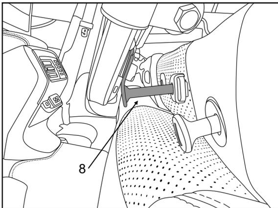
10. Insert the lateral support headrest brackets (8) into the inner headrest holes on both side of the seats.
