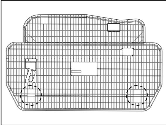
1. Locate the open apertures in the cargo barrier mesh at the bottom of the cargo barrier.
