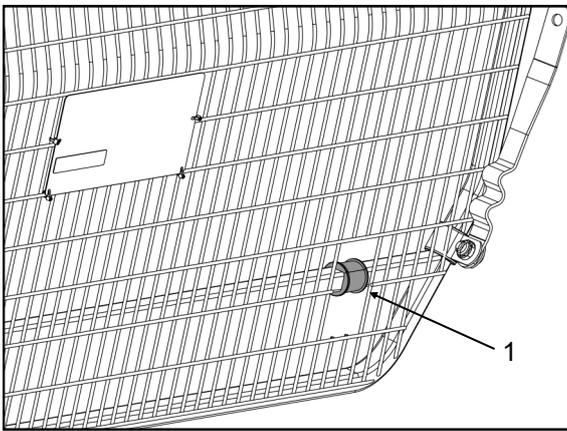
2. Place a saddle bush (1) over the cargo barrier frame as shown.
