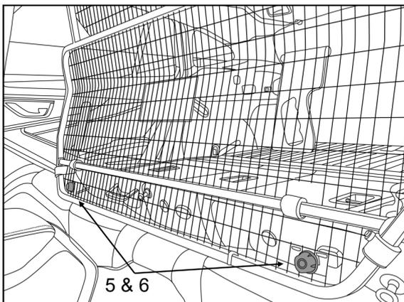
11. Support the cargo barrier mesh on the lateral support headrest brackets and fasten the mesh to the brackets using 19mm Milbolts (5) with 10mm flat washers (6) underneath the heads.
