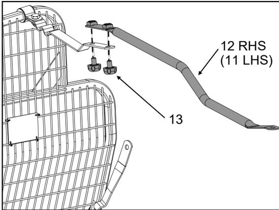
8. Fasten top tube straps to the barrier top straps as shown using 14mm Milbolts (13) (two per strap).
