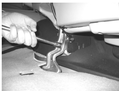
8. Using a 14mm socket driver, remove the retaining bolt. (Qty. 1) NOTE: When replacing ALL bolts must be torqued to 37Nm or 27ft. lbs
