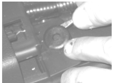
16. Remove pin clips, (1ea side) from bottom back edge of lower side trims. Using suitable trim removal tools carefully unclip the lower side trims from the vehicle.
