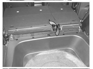
6. Unclip the floor panel located at the forward end of the cargo area. (Panel sits over the top of the forward 'D' Ring anchors)
