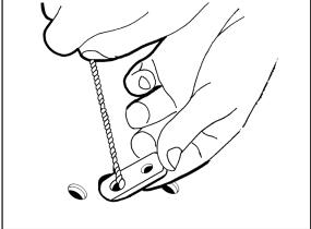
24. Whilst keeping hold of installation tool push mounting plate through 22mm centre hole in floor panel. Once plate is fully inserted, pull into position on the underside of floor panel with outer holes aligned.
