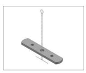
7. Place installation tool (Item 6) through centre hole in **long** mounting plate (**Item 9**). Insert mounting plate through Ø22mm hole in panel as shown. Position mounting plate behind panel with outer holes aligned.
