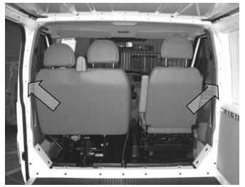
1. Locate the 3rd hexagon shaped hole down from the roof, on each rear face of the 'B' pillar as shown.
