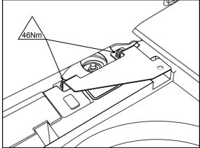
9. With the bottom brackets in position replace the flanged hex nuts removed earlier.
