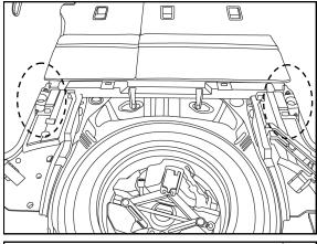
4. Familiarise yourself with the hex nuts securing the rear suspension struts in place at the sides of the cargo area.
