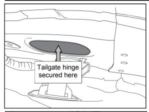
27. Familiarise yourself with the areas where the tailgate hinges are secured to the rear roof member. (oval cut outs in roof panel)
