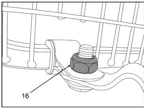
49. Place a nyloc hex nut (16) onto each of the hex screws then tighten until the strap is firm in saddle but can still be pivoted.
