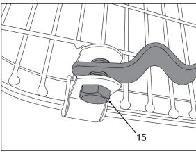
48. Place the correct strap in between the pivot saddle ends then place a hex screw (15) through the saddle and strap.
