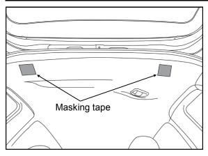
33. Affix masking tape to the cabin side of the roof lining at the approximate location of the marking pins in upper mounting brackets.
