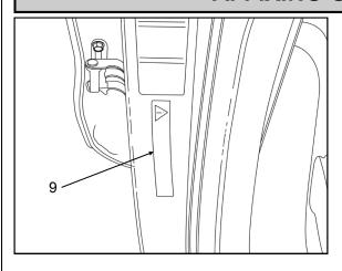
45. Clean the area inside the drivers door opening just below side airbag warning label as shown. Allow to dry then affix orange warning label (9) at that location as shown.
