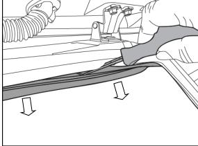
26. Using a suitable trim removal tool unclip the back edge of the roof lining allowing enough space to access the tailgate hinge securing nuts.
