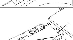
11. Screw a marking pin (4) into each of the captive nuts in bottom brackets, with just the point protruding.
