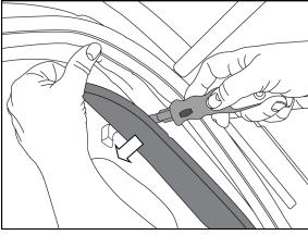
24. With the aid of a trim removal tool carefully unclip the back and top edge of the rear inner 1/4 trims. Both sides.
