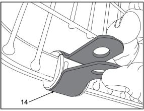
47. Place a pivot saddle (14) over each of the pivot saddle bushes then push the ends together.
