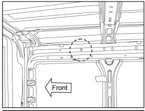
22. On the RHS (drivers side of the vehicle) locate the existing oval hole which will be used as the rearmost hole for that upper mount.
