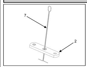
14. Place mounting plate (2) centre hole over installation tool (7) as shown.
