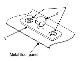
21. Place an M10 screw (5) into the centre holes to ensure correct thread alignment before fully tightening the outer screws.
