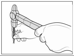
7. Centre punch the 6 marked hole positions on the floor.
