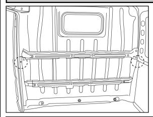
39. At the front of the cargo area about half way up the sides of the fixed bulkhead, remove the hex head screws circled. (1 each side)
