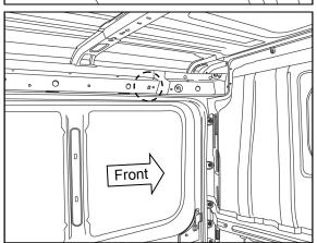
25. On the LHS (passenger side of the vehicle) locate the existing square hole which will be used as the forward hole for that upper mount.
