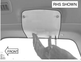
42. Repeat procedure on Drivers side (RHS) with the template in reverse. (text to back)
