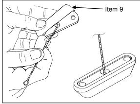
21. Fit mounting plate seal (Item 9) to mounting plate as shown.
