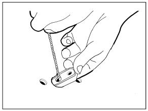
22. Whilst keeping hold of installation tool push mounting plate & seal ASM through 22mm centre hole in floor panel. Once plate is fully inserted, pull into position on the underside of floor panel with outer holes aligned.
