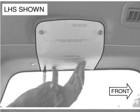
41. Whilst holding the template tight against the hard plastic trim mark through the template onto trim at indicated location.
