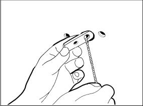
60. Whilst keeping hold of installation tool push mounting plate through 22mm centre hole in roof panel. Once plate is fully inserted, pull into position on the outside of roof panel with outer holes aligned.
