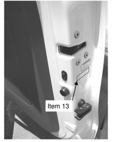
71. If the vehicle has a rear door with an interior release handle and child locks fitted please affix a 2nd warning label (Item 13) adjacent to the child lock.
