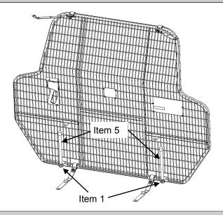
Attach support leg assemblies (Item 5) to frame brackets as shown using 24mm Milbolts (Item 1).
