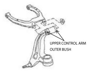
The camber can be adjusted depending on the kit you have purchased. Check on initial wheel alignment spec to see what setting is required.
