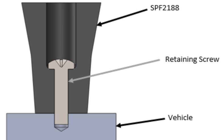
Figure 2: Installation diagram of SPF2188
