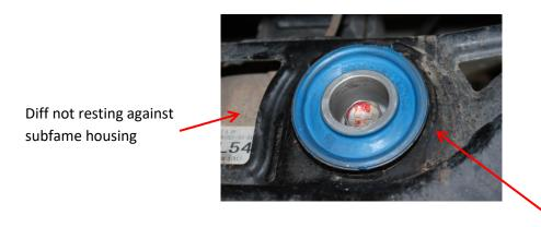
Need to check here to be sure bush is fully into housing
