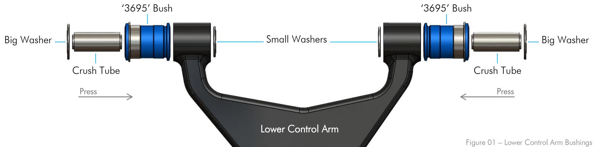
Figure 01 – Lower Control Arm Bushings
