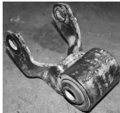
Rear, Spring Shackle with factory bushes (LEFT) and polyurethane bushes (RIGHT)
