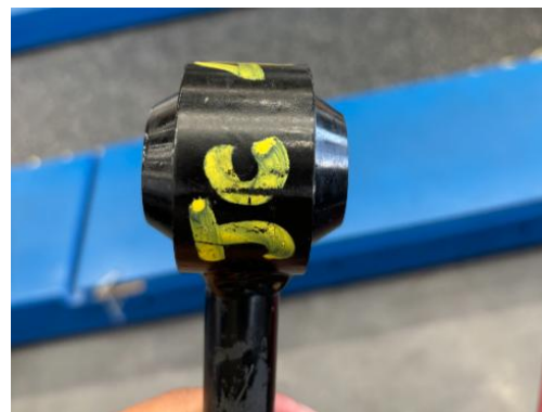
Figure 2: New polyurethane bush in arm
