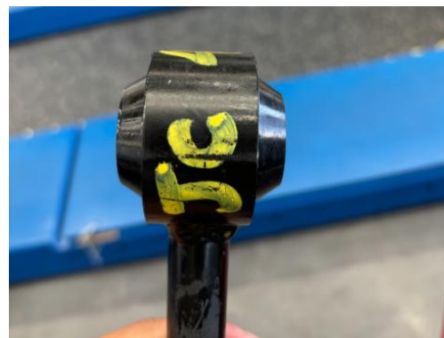
Figure 2: New polyurethane bush in arm
