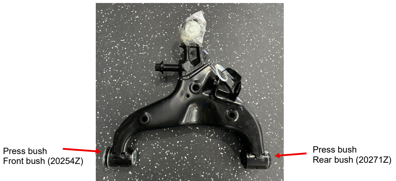
Right hand arm shown (washers on rear bush not shown)
