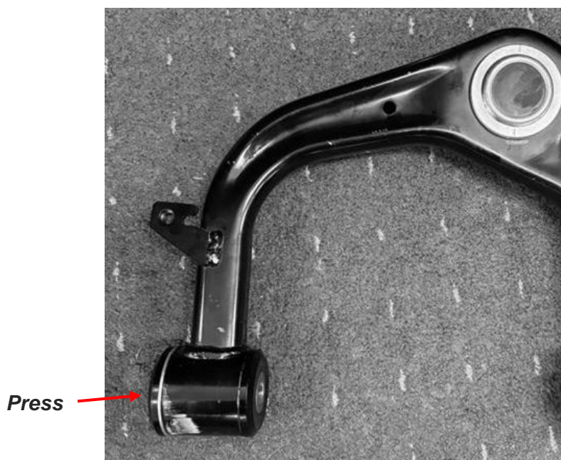
Front Side of RHS FUCA Shown.
