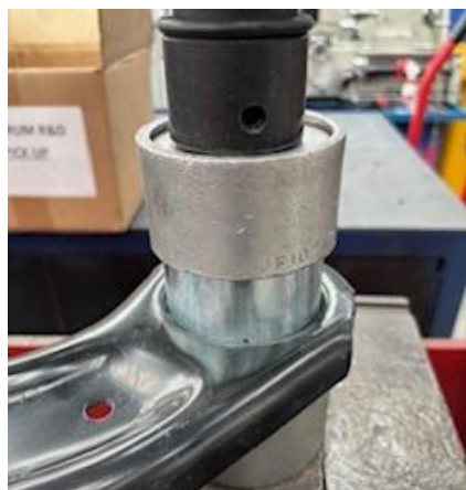
Figure 1: Press tools to push in shell
