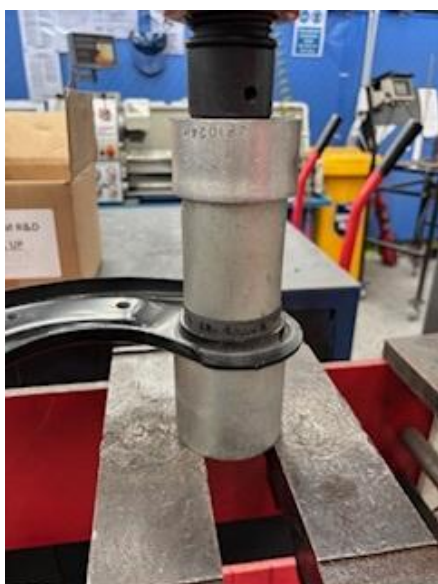
Figure 1: Press tool assembly to push bush out
