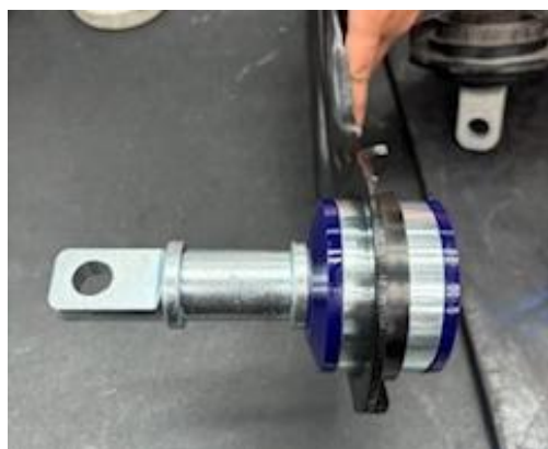
Figure 5: Blade tube to be pressed into bushing
