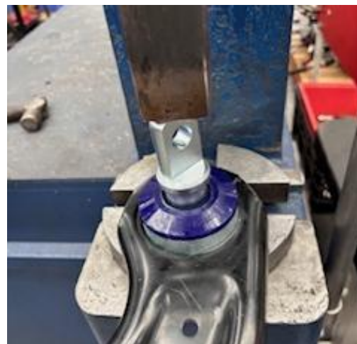
Figure 6: Blade tube pressing into bush in arbor press
