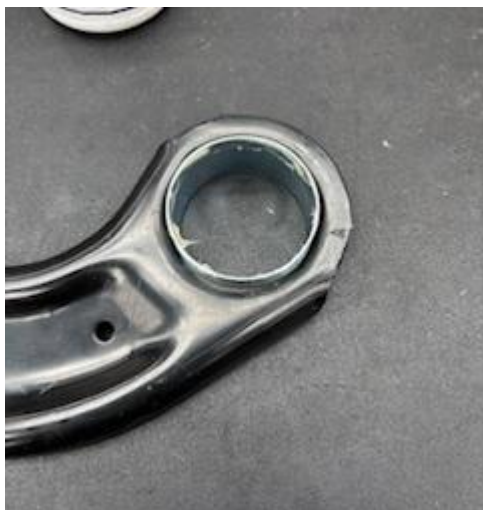
Figure 4: Grease to assist with pushing in new bushing
