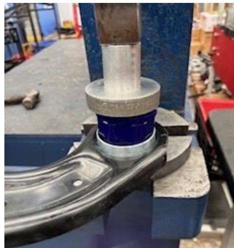
Figure 3: Press tools used to push new bushing into shell
